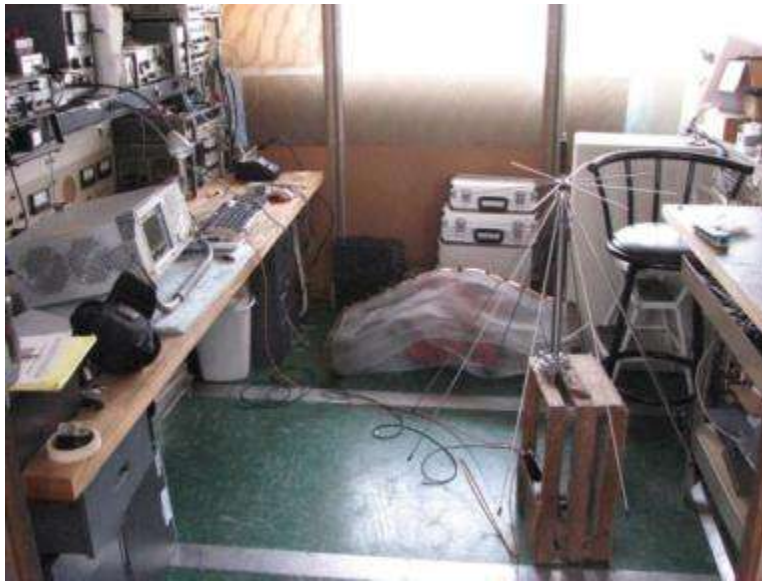
Figure 7. RFI measurements of the generator
