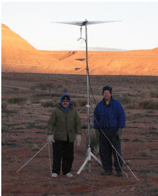
Figure 2. CLP5130-2 UHF Log Periodic Antenna from Creative Design Corp. with a frequency range of 105-1300MHz, a gain of 11-13dBi, and horizontal polarization.
