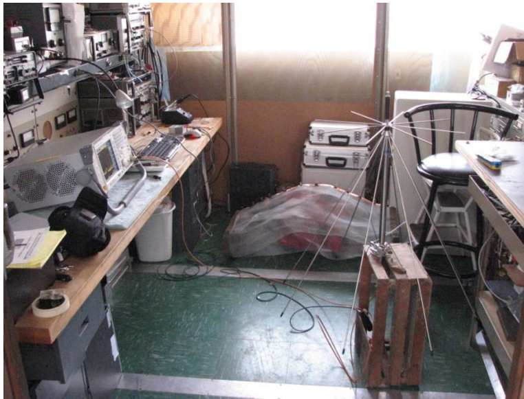
Figure 7. RFI measurements of the generator
