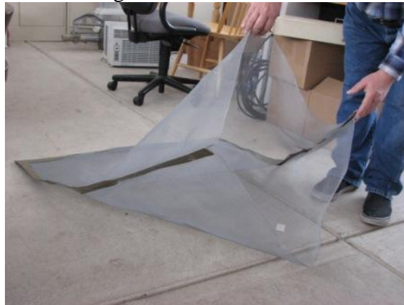
Figure 6. Photo graph of a “screen bag” for RFI shielding.
