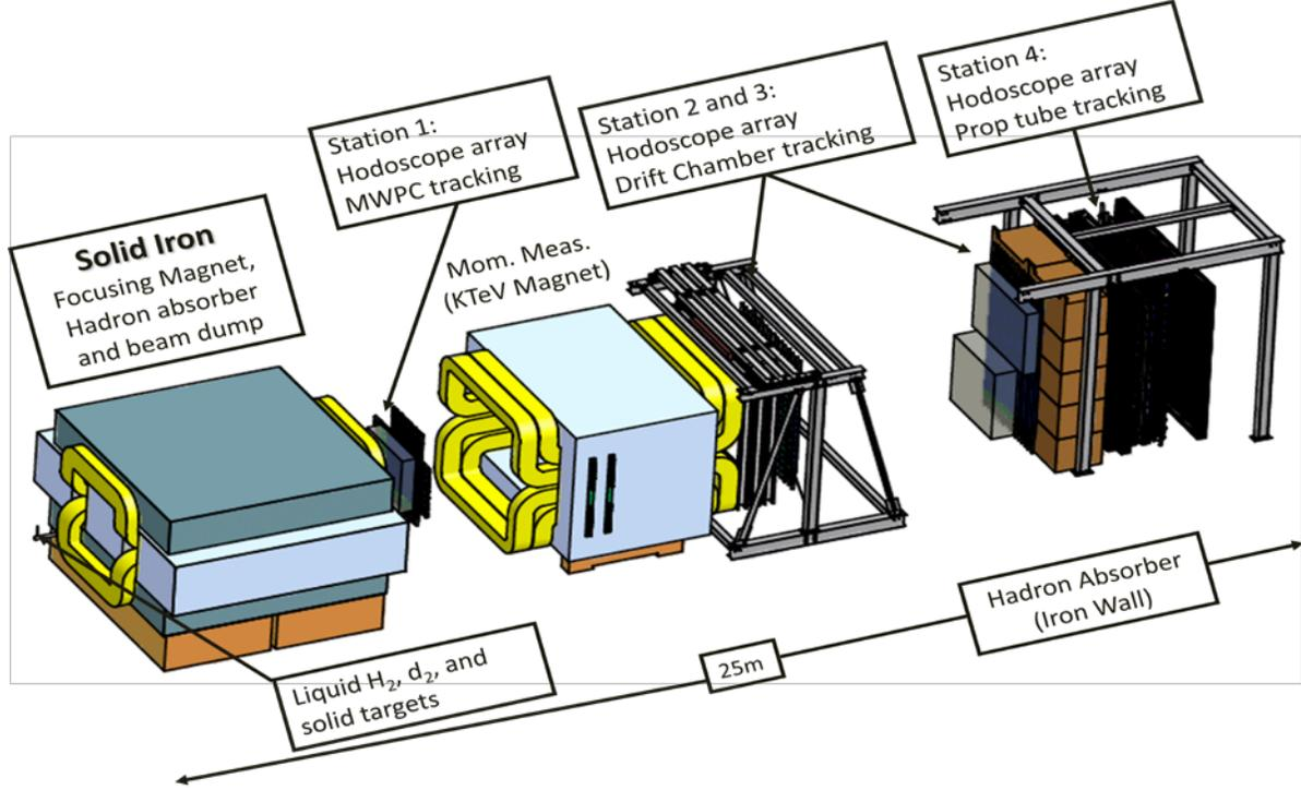
**FIGURE 4.** Schematic layout of the E906/SeaQuest Drell-Yan Spectrometer.
